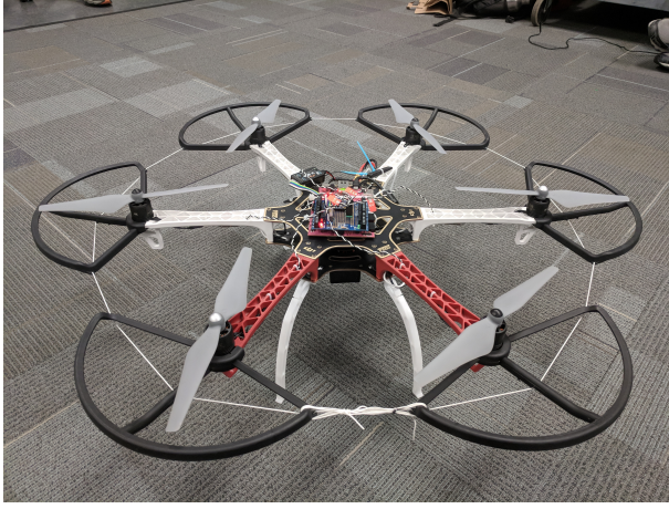
Fig. 6. Fully-assembled PynqCopter UAV including batteries, sensors, controller, propeller guards, and propulsion system.
