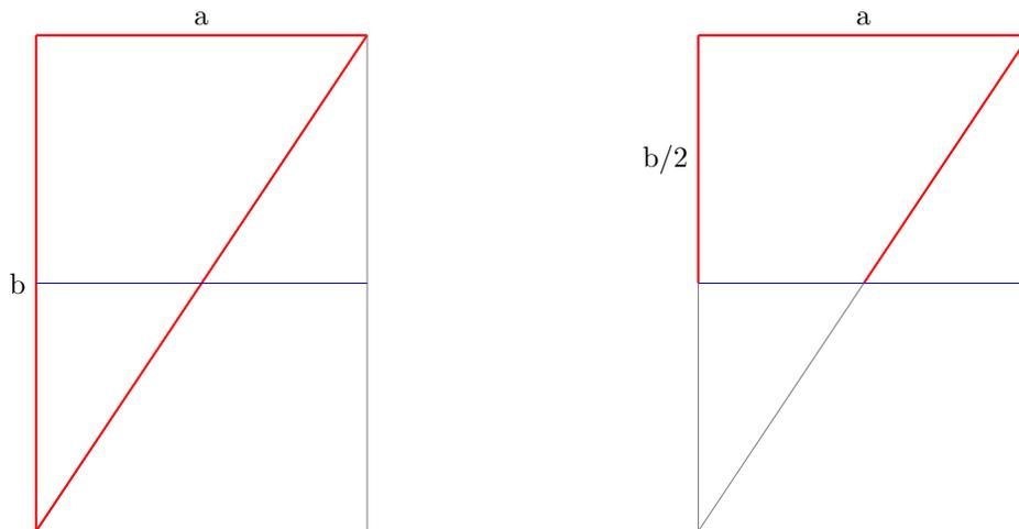
Figure 2: Triangle with Equal Area to Rectangle
